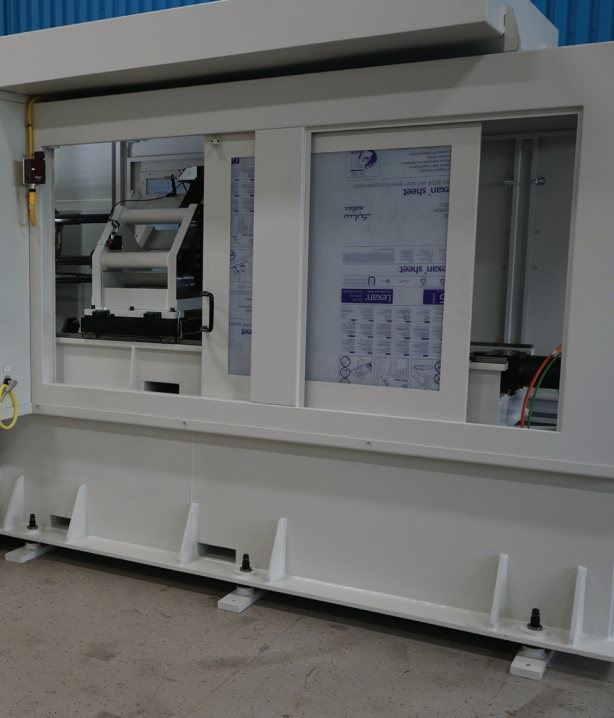
Brush and gauge crank bore; a stand-alone station gantry loaded. Photos courtesy of Adesco Engineering.
