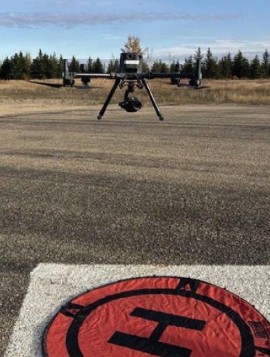
Drones equipped with non-destructive testing (NDT) payloads are invaluable tools to catch problems before they happen along Alberta's extensive network of powerlines.
