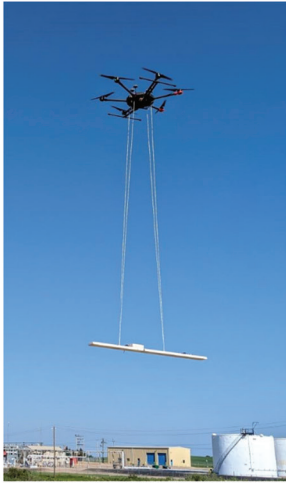
RPAS with EM and methane sensor, with EdgeFuse, in flight
